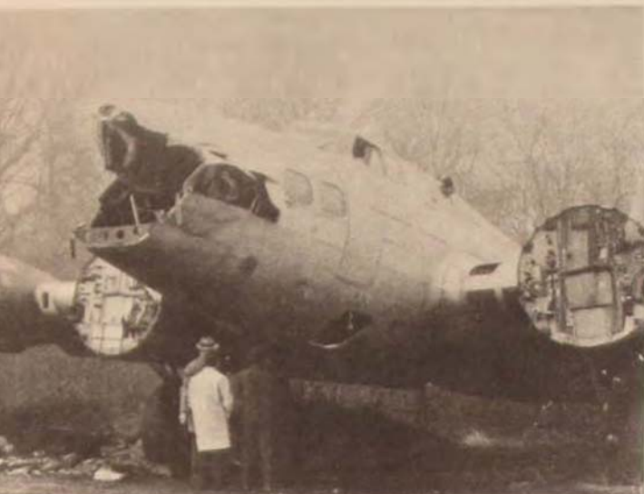
Hardly recognizable even as a B-17 (the result of various postwar modifications for civilian use in Sweden, Denmark, and France as well as subsequent nose damage), Shoo-Shoo Baby was given to the U.S. Air Force by France. Recovery began by dismantling her to go home.
